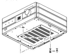
The feet can also be attached to the back-side holes. If the front side of the device is not stable, attach the feet to the back-side holes.
