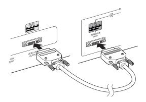
Do not connect a computer monitor or the like to the terminal. It will cause a malfunction.
